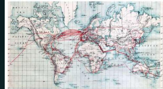
Fig. 2. Cable map of the world, 1901, from W. Clouston-Thorne, A.B.C. Telegraphic Code, 5th ed., London, U.K.: Edes Fisher & Co., 1901, courtesy of Bill Duma. The dashed lines in the Pacific represent cables then in the planning stages; the one from Canada to Australia and New Zealand was completed in 1902, while the one from California to Hawaii was laid at the end of that year and extended to the Philippines in 1903.
